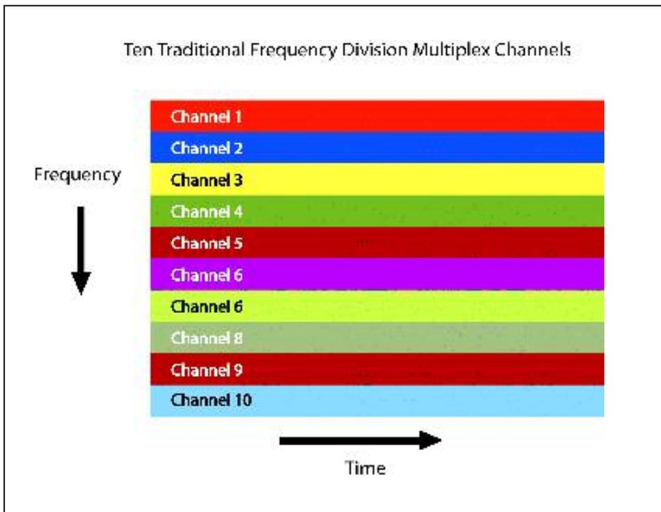
**Figure 2. Ten Separate Frequency Division Channels**
